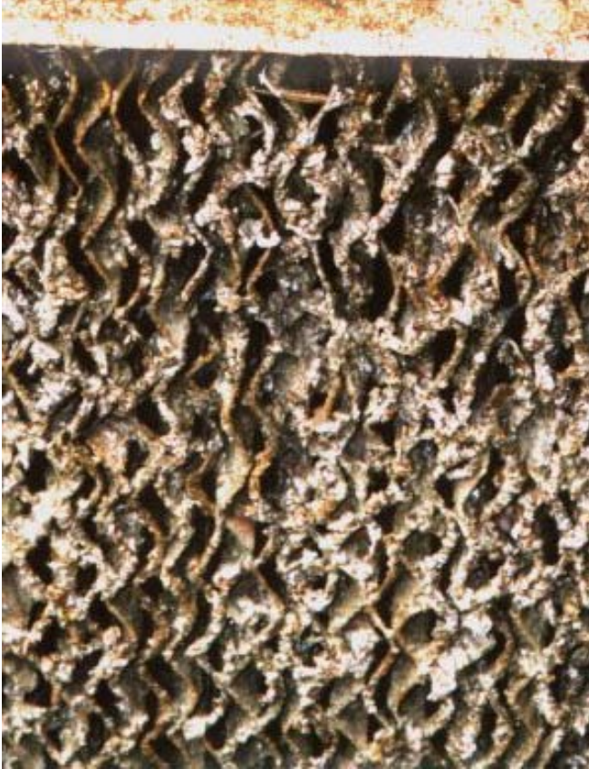
Figure 2: Photos of evaporative cooling media. LEFT (BEFORE Zeta Rod installation) - Significant build-up of slime and scale interferes with wetting of media and impedes air flow. RIGHT - 6 weeks after installation of the Zeta Rod system, layers of fouling and scale swelled and loosened, and the media was restored to clean condition by washing with a low-pressure garden hose.
