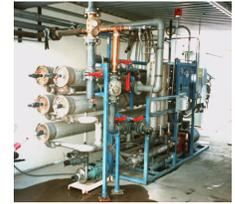
**INTRODUCTION** Reverse Osmosis ("RO") machines are now widely used to produce high-purity water for beverage, semiconductor, and other products and processes that require particle- and bacteria-free water. Water is pumped into the machine at high pressure, where it is forced through the membranes, leaving behind particles such as bacterial cells and suspended materials.
