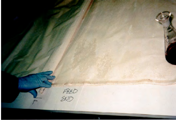
Figure 1. View of concave side of Leaf 2 (on right) and convex side of Leaf 1 (on left). Product water tube runs from lower left to top center. The feed end of the leaf is at the bottom (as marked on the autopsy table). The vexar netting lies on top of Leaf 2. The darker beige blotches are the accumulations of salt on the leaf.
